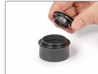
This image shows how the glasspath corrector is inserted into the optional T-2/2"-adapter. The black plastic ring covers the thread of the GC, so that it will be centered in the adapter.
