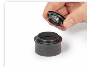
This image shows how to insert a glasspath corrector into the optional T-2/2" adapter. The black spacer ring fits onto the thread of the glasspath corrector and centres it in the nosepiece.
